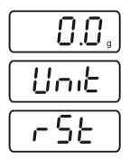
⇒ In weighing mode keep the **PRINT** key pressed until **[Unit]** appears.
